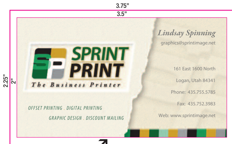
Incorrect - NO BLEED
